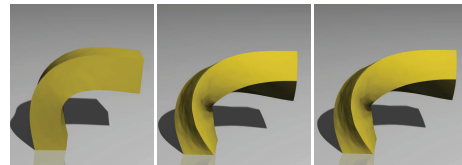
Figure 14: Elastic bar guided by example with coupled twisting and bending, using different number of eigenfunctions. 2 eigenfunctions (left) fail to capture the twisting, while 14 eigenfunctions (middle) are sufficient to capture both bending and twisting. Increasing the number of eigenfunctions to 30 generates similar result (right).
