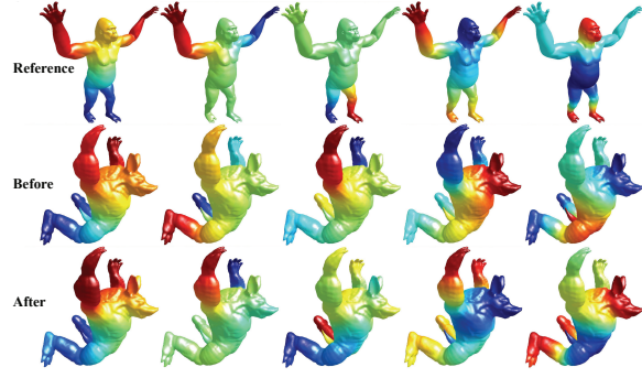
Figure 2: The eigenfunctions of a deformed armadillo are registered with respect to the eigenfunctions of a gorilla. After the registration, the eigenfunctions between the shapes are consistent. Hot and cold colors represent positive and negative values, respectively.
